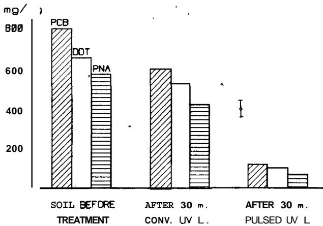
**FIGURE 7.** Reduction of PNA's, PCB's and DDT from the soil, placed into a 18 cm by 5 cm tray in 1.5 cm thick layer. The lamp was 5 cm from the soil and had a parabolic UV reflector. (1)—Initial concentrations. (2)—Reduction after 30-min. treatment with a medium pressure mercury lamp at 60wt/cm load. (3)—reduction after 30 min treatment with UV pulsed lamp at the same loading.
