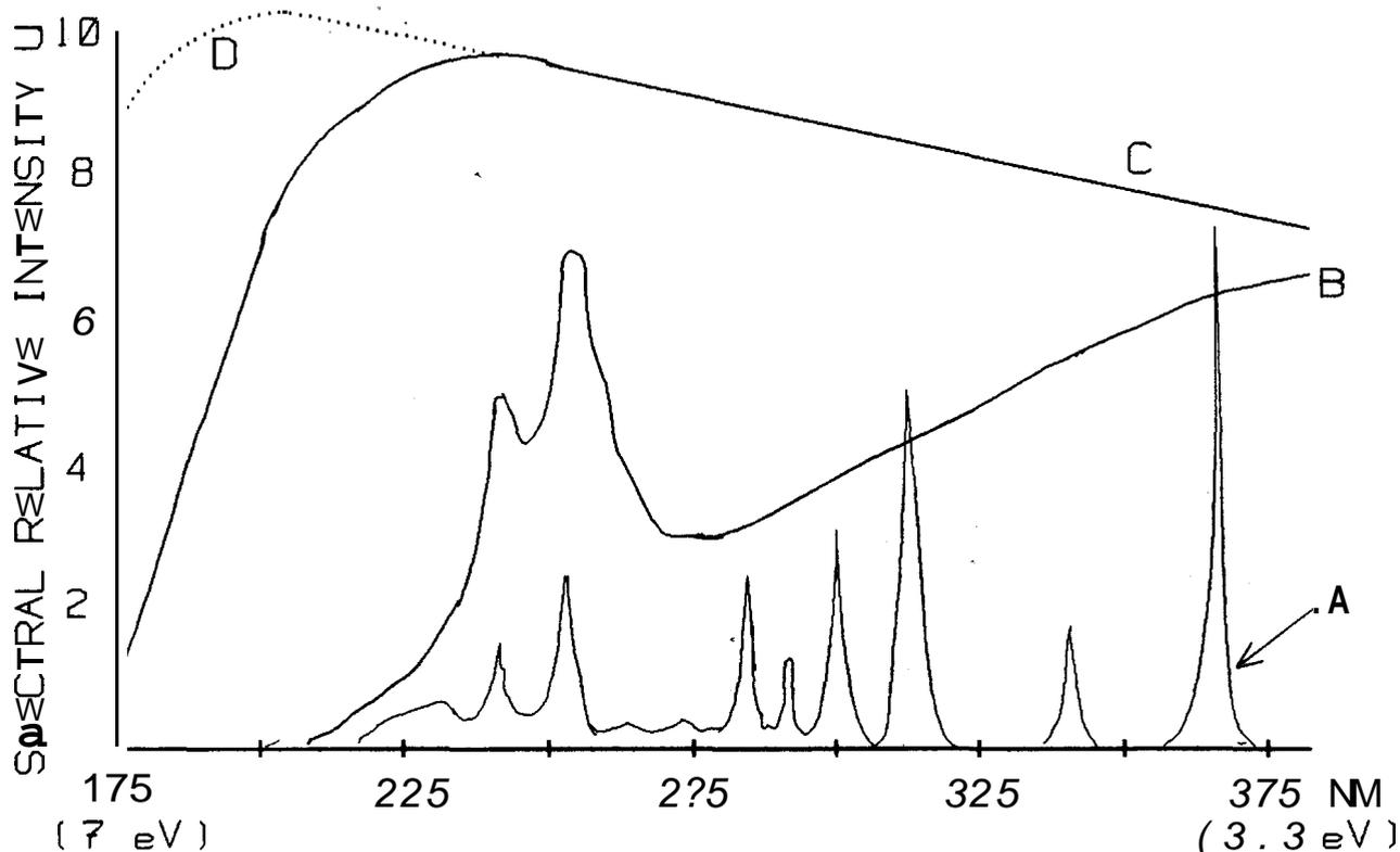
FIGURE 1. Spectral distributions in the region from 175 nm to 375 nm for four UV sources (A, B, C and D) in relative units  $U$ . Corresponding maximum and minimum photon energies for the region are given in eV ( $1 \text{ eV} = 1.6 \cdot 10^{-19}$  Joules,  $1 \text{ nm} = 10^{-9} \text{ m}$ ).
