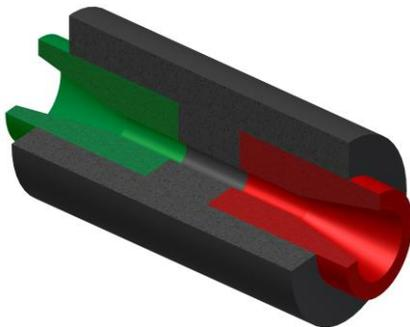
Red- HV electrode, green-ground, black-insulator. Electrodes often electrostatically focus el. fields by its shape (as above) to increase power density in volume discharges.
